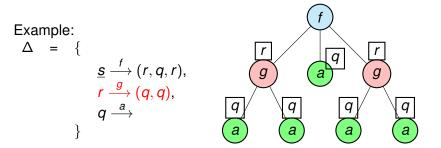
Finite Non-deterministic Tree Automaton (TA):  $A = (Q, \Sigma, \Delta, F)$
