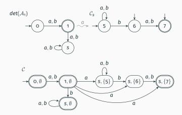
**state of** C: state of  $det(A_1)$  + states of current instances of  $C_2$  **final states:** C accepts when all current instances of  $C_2$  accept
