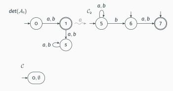
**state of**  $\mathcal{C}$ : state of  $det(\mathcal{A}_1)$  + states of current instances of  $\mathcal{C}_2$  **initial state of**  $\mathcal{C}$ : initial state of  $det(\mathcal{A}_1)$  + no running instance of  $\mathcal{C}_2$
